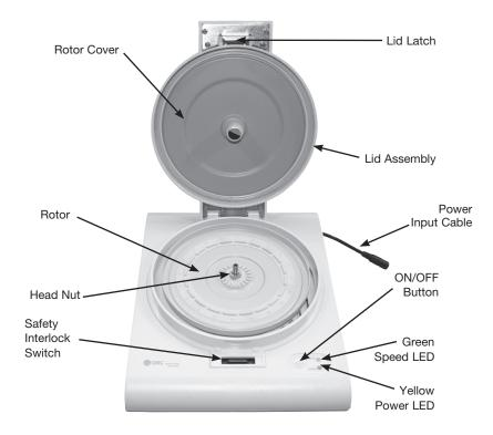
Figure 2-1. Features and Controls of QBC Capillary Centrifuge.
