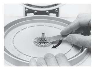
Figure 3-5. Tightening Rotor with Head Nut Wrench
