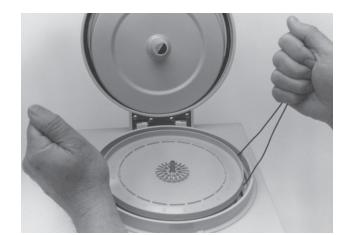
Figure 9-1. Prying Rotor From Motor Shaft with Removal Wire.
