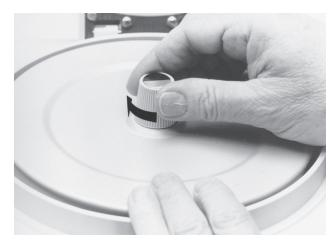
Figure 4-4. Tightening Knob of Rotor Cover.
