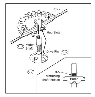
Figure 3-4. Installing Rotor Assembly.
